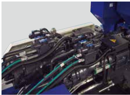
Compact injection units Two single coaxial injection units provide stable and accurate injection control
