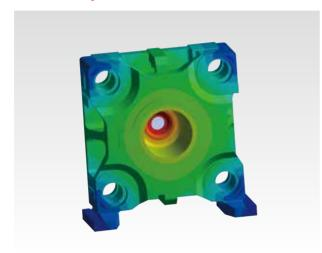
The newly designed platen is specially engineered for packaging products. The finite element software analysis shows that the average deformation is reduced by more than 30% compared to a normal hydraulic injection molding machine, effectively improving the precision of the products.
