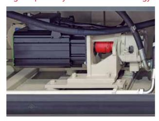
The new servo motor with low inertia is equipped with high speed hydraulic pump to provide better acceleration response performance. It provides stable and reliable hydraulic driving force for injection, opening and closing mold and other actions. The perfect combination of economy and performance.
