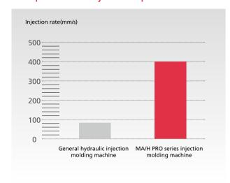
Supported by new servo motors and redesigned gear pumps, the maximum injection speed of the MA/H PRO is more than 400 mm/s. Through optimized hydraulic output, the injection process is stable and controllable.
